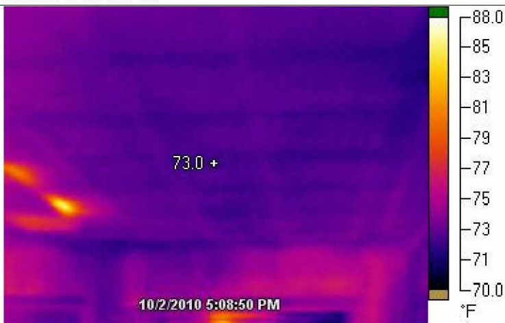
The ceiling got cold when depressurized, indication that outside air can travel under the insulation.
