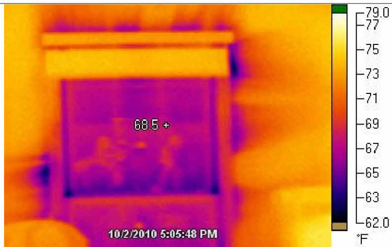
Air leakage at the window is shown by the dark spots that fan out from the window trim. Most
