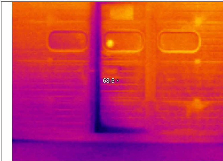
Air leakage around the door.
