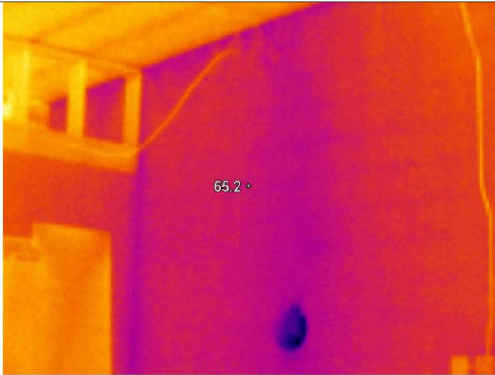
The open hole to the old chimney.
