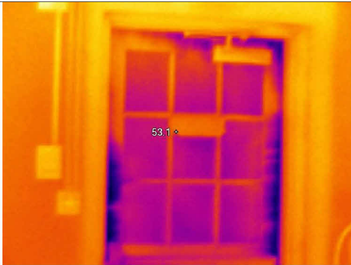
Typical exterior door with air leakage around it.
