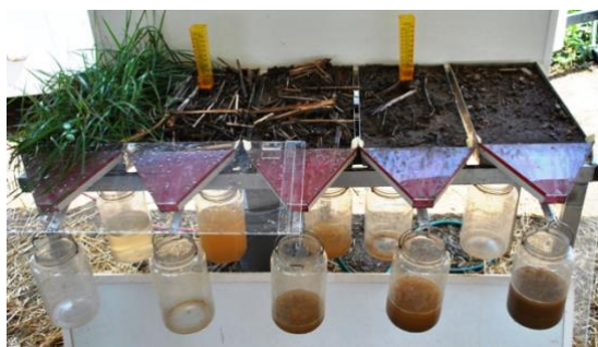
Rainfall Simulator showing water runoff (jars in front) and infiltration (jars underneath soil) from different soil management types (Source: Benton James, Madison County Soil Conservation District, TN)
